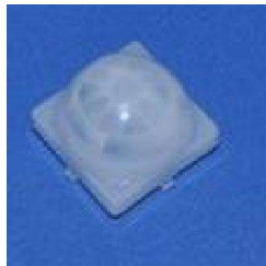
Model: 023100 Size: 23.4*23.4* 18.9 Focal: 10.5mm Angle: 120 ° Distance: 10m
