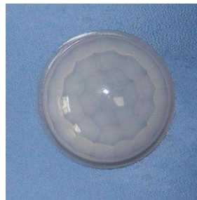
Model: 8003-2F-X Size: 25.5* 12.3 Focal: 10.5mm Angle: 120 ° Distance: 10m
