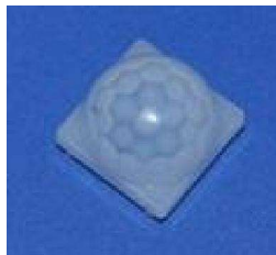
Model: 8002-2 Size: 23.3*23.3* 14.8 Focal: 10.5mm Angle: 110 ° Distance: 11m
