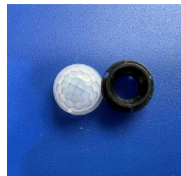
Model: YY-1508 Size: Ø16.8 *12.05 Focal: 7.5mm Angle: 360 ° Distance: 2.5m
