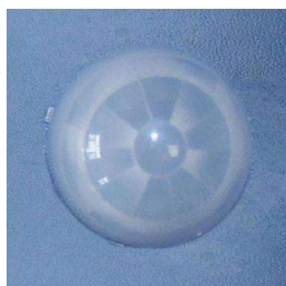
Model: 8003-4 Size: \varnothing 23.2 \times 18.8 Focal: 10mm Angle: 120 ° Distance: 10m
