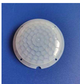
Model: YY-5316-F Size: \Phi 53* 11.6 Focal: 20mm Angle: 360 ° Distance: Dia. 12m ceiling mounting 6m
