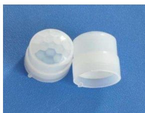
Model: 8308-6 Size: 13.6 * 15.5 Focal: 9.6mm Angle: 90^\circ Distance: 8m
