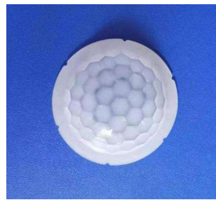
Model: 8603-6G Size: Ø38.8 Focal: 17.5mm Angle: 360 ° Distance: 14m
