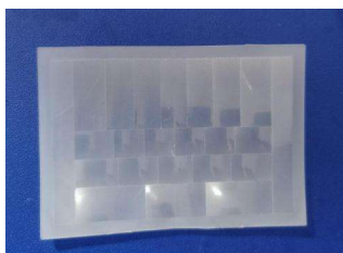
Model: YY-EWA-V3 Size: 42.6 *61 Focal: 30.5mm Angle: 140 ° Distance: 15m
