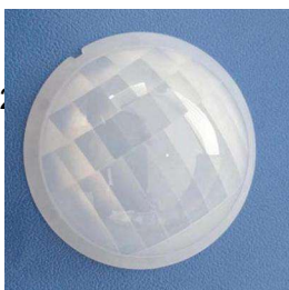
Model: YY-3015 Size: \varnothing 34 \times 15 Focal: 15mm Angle: 135^\circ Distance: 12m
