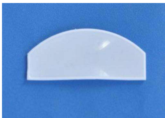
Model: SIR 650 Size: 46*20 Focal: 30mm Angle: 15 ° Distance: 12m
