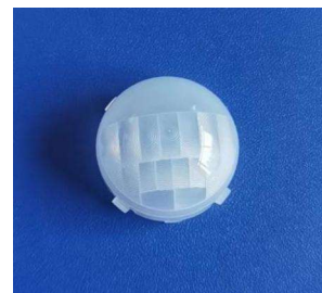
Model: YY-2311 Size: \varnothing 12.5 Focal: 11mm Angle: 120 ° Distance: 10m
