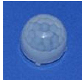
Model: 8003-1 Size: \varnothing 22.7 \times 18.6 Focal: 10.5mm Angle: 100 ° Distance: 10m
