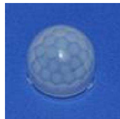
Model: 8005-2 Size: \varnothing 23*19.7 Focal: 11mm Angle: 120 ° Distance: 10m
