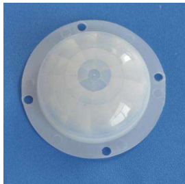
Model: 8605-3W Size: \varnothing 43.6* 11.4 Focal: 15mm Ceiling :2.5M Angle: 360 ° Distance: Dia.: 10m
