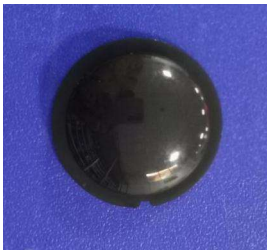
Model: YY-01 Size: \varnothing 21.3 \times 6.1 Focal: 8mm Angle: 120^\circ Distance: 8m
