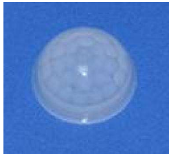
Model: 8003-2F Size: \varnothing 25.3*12.5 Focal: 10.5mm Angle: 120 ° Distance: 12m
