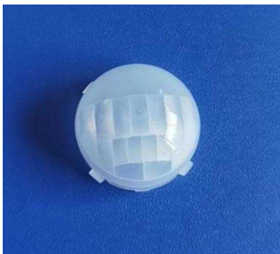
Model: YY-2311 Size: Ø23.22* 12 Focal: 11mm Angle: 120 ° Distance: 10m The pattern-free area is facing down and placed 1.2m away to prevent pets.
