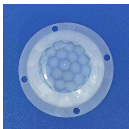
Model: 8605-3G Size: \varnothing 44.5 \times 12.2 Focal: 15mm Ceiling mounting 3M Angle: 360 ° Distance: Dia.: 12m
