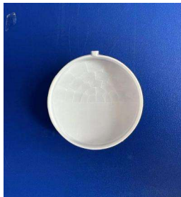
Model: YY-RG01 Size: Ø39.8*7.7 Focal: 12mm Angle: 120 °-130 ° Distance: 8m
