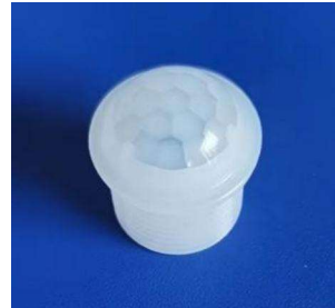
Model: YY-2311 Size: Ø23.22* 12 Focal: 11mm Angle: 120 ° Distance: 10m The pattern-free area is facing down and placed 1.2m away to prevent pets.
