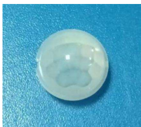
Model: 13120F-5 Size: \Phi 13.7 * 6.6 Focal: 6mm Angle: 120^\circ Distance: 7m
