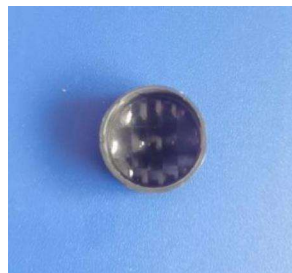
Model: ZMD-2020-8 Size: Ø20*9.2 Focal: 5mm Angle: 120 ° Distance: 5m
