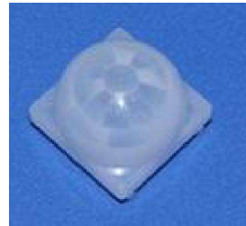
Model: 8002-2W Size: 23.3*23.3* 14.7 Focal: 10.5mm Angle: 120 ° Distance: 12m
